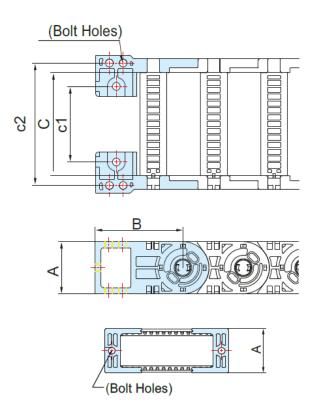
= C-25 = C+15 A = 82 B = 156 C Inside measure = Model Hole size = M10
